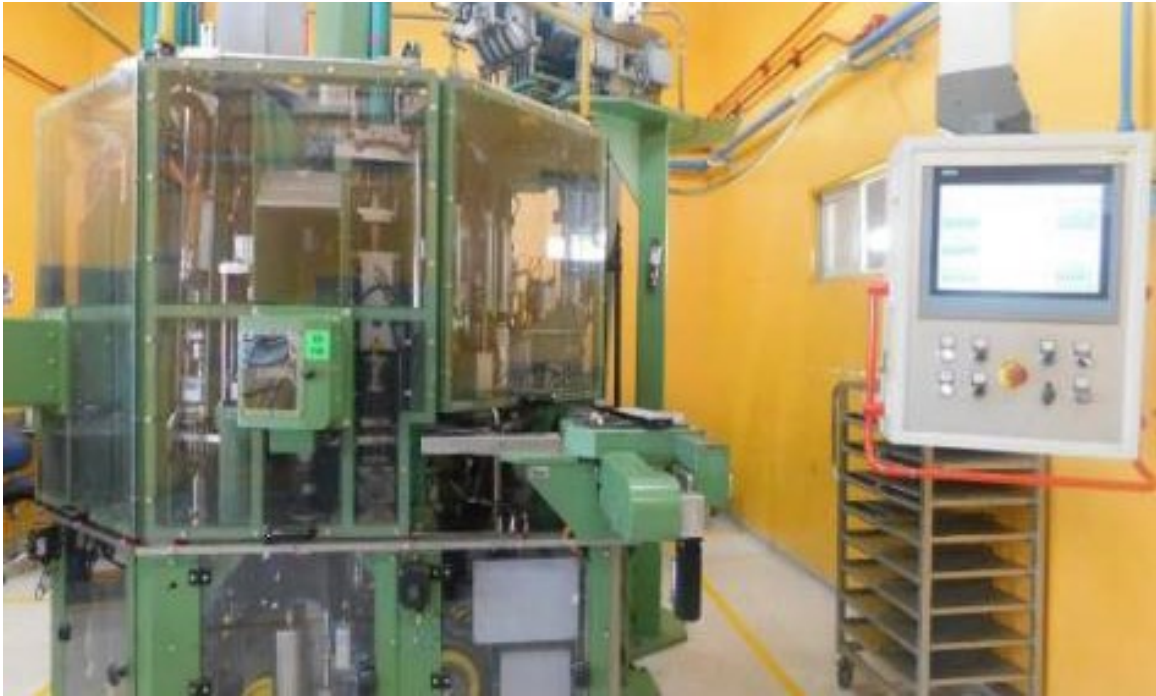
Element filling and pressing machine prior to the event
